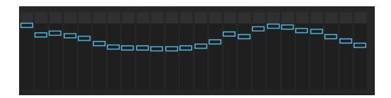
The Band Gain Multi-Slider lets you individually set the gain for each filter band. It functions very much like a graphic EQ, allowing you to sculpt the frequency response of the vocoder output.
