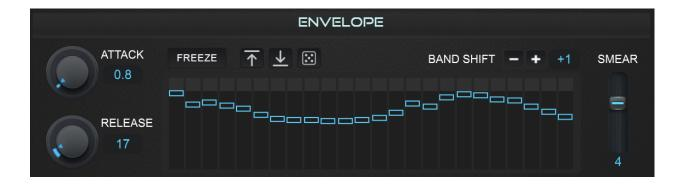
The Envelope controls let you configure the volume level of each filter bank independently, and also how the filter banks respond to the detected amplitude of audio input (e.g. your voice).
