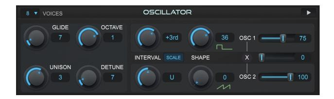
The Oscillator controls let you configure Auto-Tune Vocodist's powerful built-in 8-voice, dual-oscillators. When the Source control is set to Oscillator, these oscillators function as the synthesis channel input into the vocoder.
