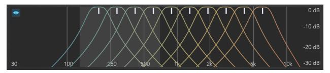
The Filter Graph gives a real-time visual representation of the frequency response of the analysis and synthesis filter banks.
