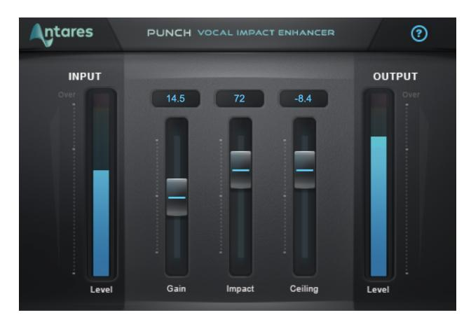
**Punch** is a dynamics processor that gives your vocals more dynamic impact. It provides a combination of compression, gain, limiting, and overload protection with an interface designed for speed and simplicity.
